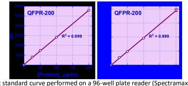
*Left*: standard curve performed on a 96-well plate reader (Spectramax M2); *Right*: correlation plot obtained on handheld fluorimeter
